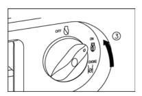
After the engine starts, warm up the engine until the engine does not stop when the 3 in 1 switch is returned to the "ON" position (3).
