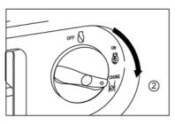
Turn the 3 in 1 switch to "CHOKE" (2)
