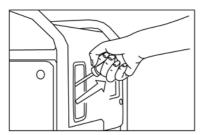
Firmly grasp the recoil handle and pull slowly until increased resistance is felt. Pull rapidly up and away.
