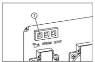
TIP: If the engine stalls or does not start, turn the engine switch to "ON" and then pull the recoil starter. If the oil warning light flickers for a few seconds, the engine oil is insufficient. Add oil and restart.
