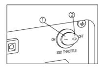
When the ESC switch is turned to "OFF", the engine runs at the rated (3100 r/min) Regardless of whether is a load connected or not.
