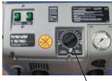
Thermostat with rotary control switch
