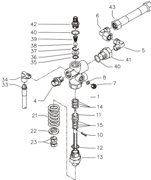
Safety valve for heating coil
