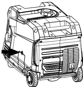
2. Clean area around oil fill/drain plug and remove plug.
