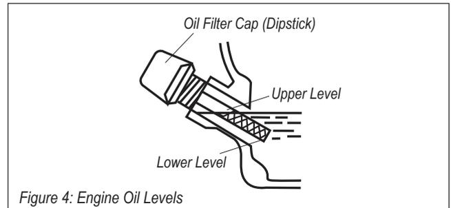
4. Do not overfill, if oil level is too high, oil will drain out through the fill plug.
