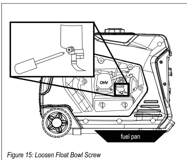
Figure 15: Loosen Float Bowl Screw
