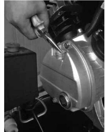
3. Locate the plastic dust plug in the oil breather hole and remove it to expose the oil breather hole.
