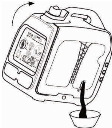
Figure 14: Carefully tip inverter so oil flows into oil pan
