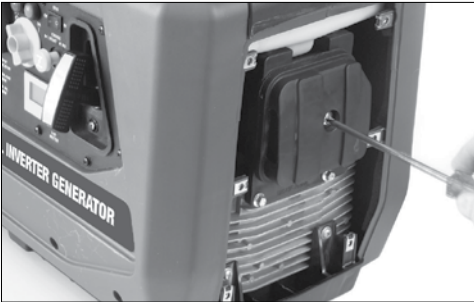
Figure 16 – Removing the Air Filter Cover
