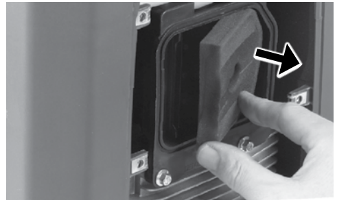
Figure 17 – Removing the Air Filter Element
