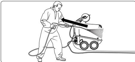
Bear in mind that during cleaning tasks with a high-pressure water jet a significant recoil at the lance arises (see technical data on page 2).
