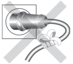
Do not damage the power cable or repair it incorrectly!
